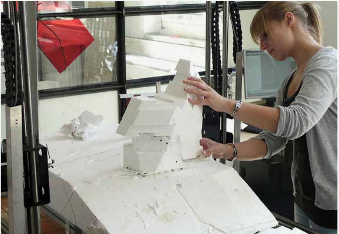
Working with the computer-controlled hot-wire cutting machine.
