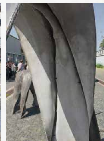
4a–b IMD students, Concrete Canvas , 2015, led by Daniel Büning. Prototypes, cement-impregnated fiber-reinforced fabric.
