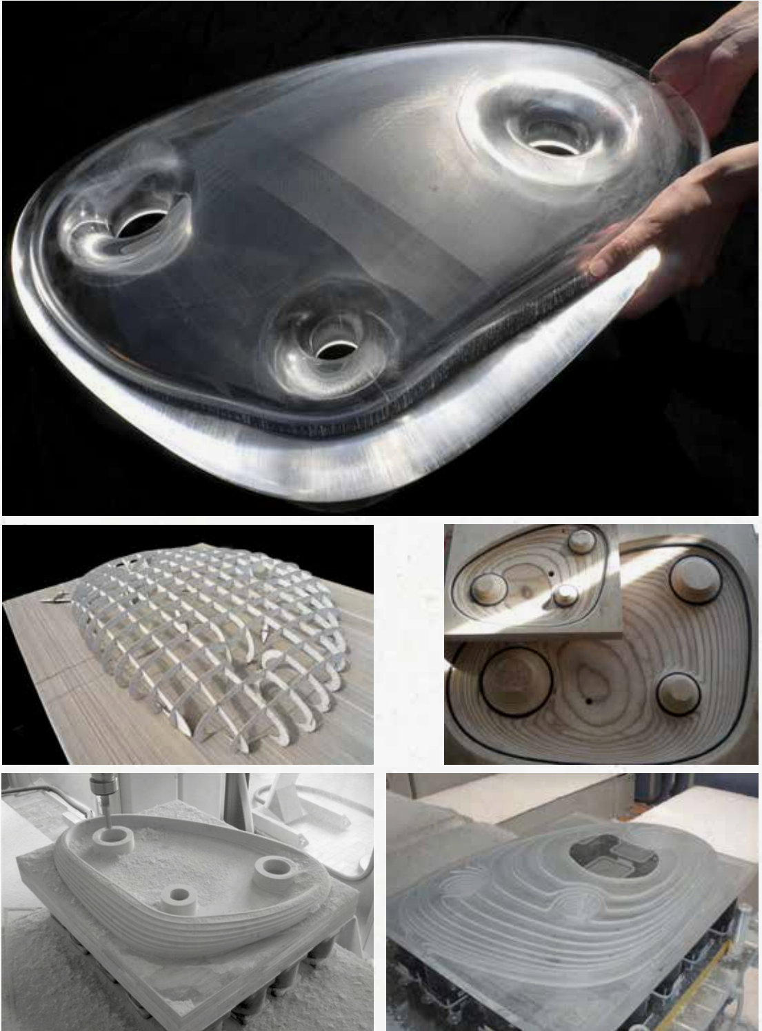
Ulrike Knauer and Robert Uhl: A Design for an Airplane Hangar. CNC milling and laser cutting models.
